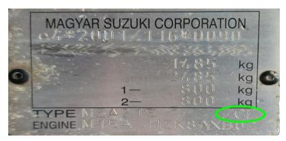
Suzuki paint codes are usually 3 digits, and can be either all letters (usually including a Z) or a mix of letters and numbers – for example: **ZWP, ZCE, Z7T, 26U**
